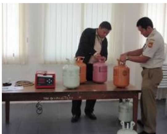
Identification of suspicious refrigerant. Goods seized by Customs Office in Tanjung Balai Karimun Indonesia October 2007. Photo: Astutie Widyarissantie; April 2008, National Ozone Unit, Ministry of Environment of Republic Indonesia"
